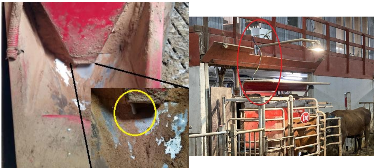
Figure 1: Sniffer equipment at Assendrup. Gas tube installed in feed through (Left) connected to the AMS (Right).
