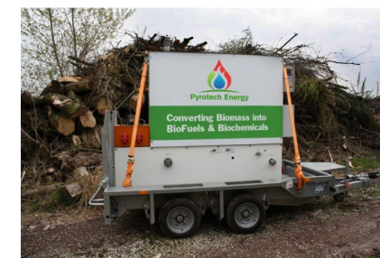
Mobile Pyrolysis Plant to Convert Biomass and Agriculture Residue to Bio Fuels.
