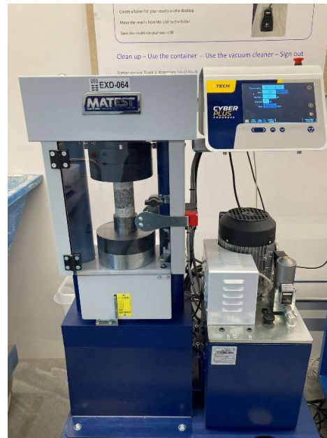
Figure 3: MATEST Cyber Plus Progress used for compressive test measurements
