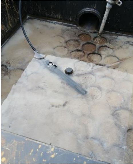
Figure 12. Insoluble \text{Al}(\text{OH})_3 flocs at the surface of the reactive filter observed on the 15-02-22.
