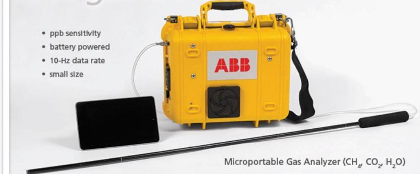
Microportable Gas Analyzer ( $\text{CH}_4, \text{CO}_2, \text{H}_2\text{O}$ )
