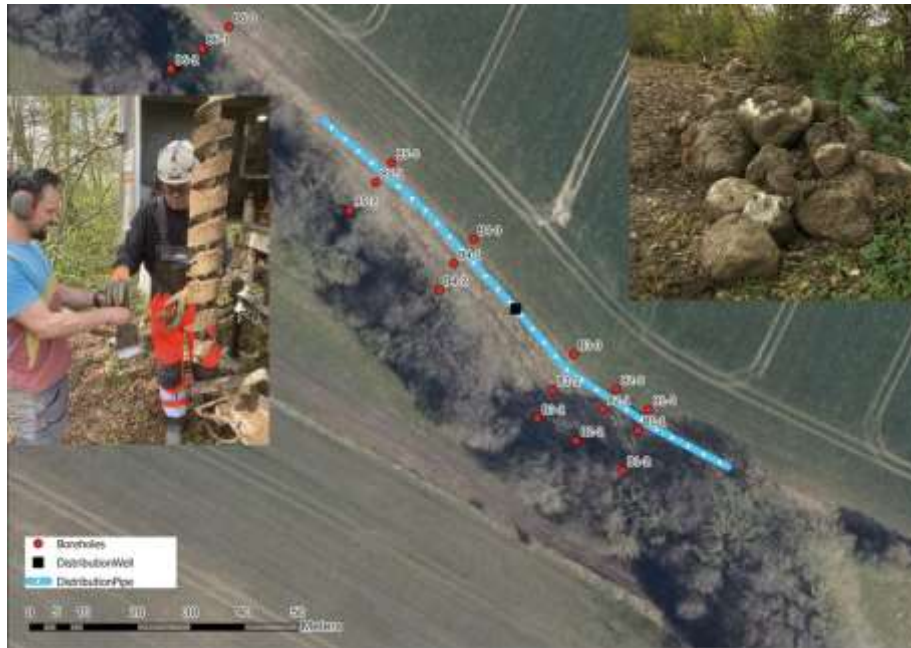
Fig. 8 The saturated buffer zone Bondesvad fully instrumented in May 2022. Large rocks found in about 1 m soil depth and soil sampling for texture description.
