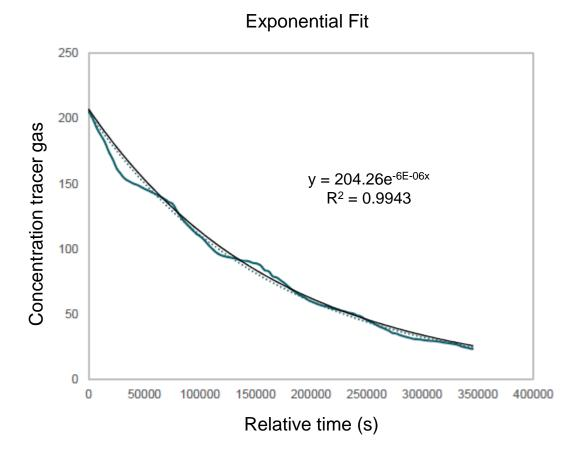
The air exchage rate is determined from the general mass balance for the tank:
